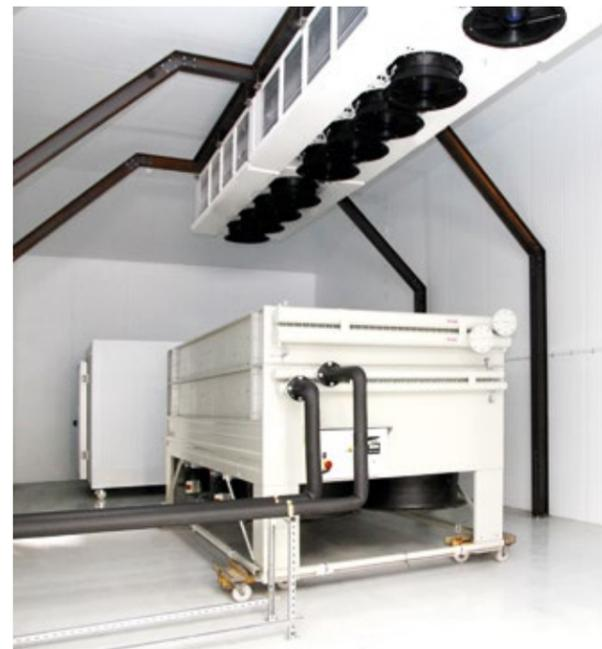
Unit under test in large calorimeter room
